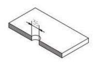
Mark hole in benchtop at desiredposition and drill a 35mm hole.
