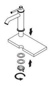
2. Install the basin mixer by fixing the basin/benchtop between the mixer andthe rubber seal, locking plate and nut.
