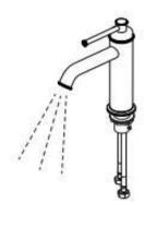
Attach the flexible hoses to the water supply and tighten. Test and commission.
