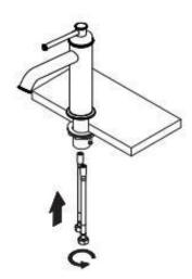
Connect the hot and cold flexible tails to basin mixer. The cold supply must be on the right and the tails should only be hand tightened into the mixer body.
